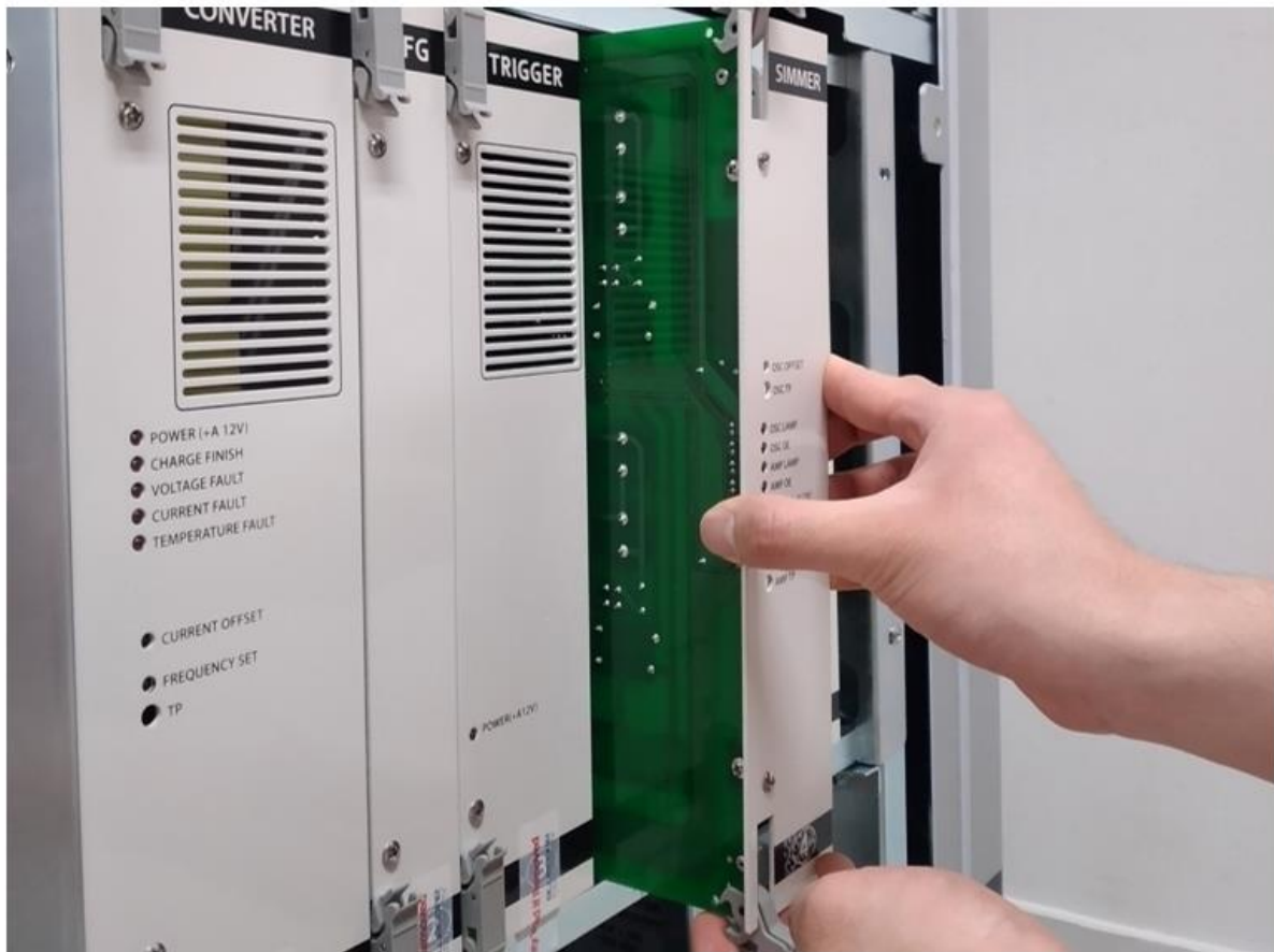
Slot-type electrical system for easy and fast maintenance
